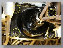
the train. It is surrounded by other hardware making access difficult but particularly the position of the Absolute Position Reader (APR) which is a large boss in the centre of the fourbolt flange.
