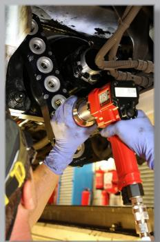
Upper bolt using one of the short reaction orientations
