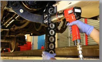
Lower bolt using long reaction
